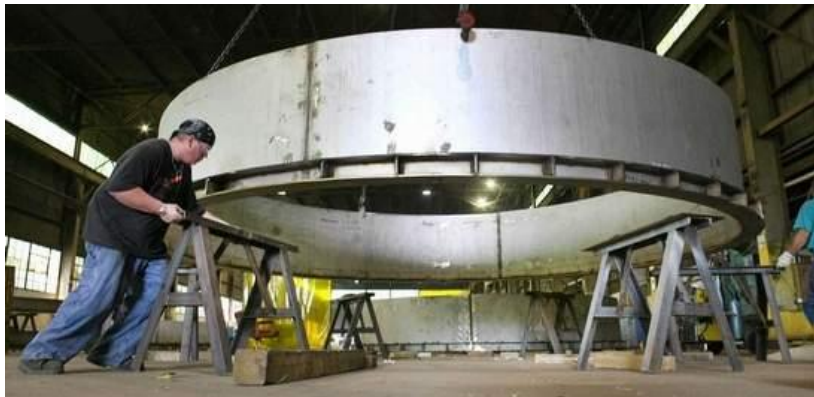
Matt Bartow constructs a tank earlier this month at Edgemoor's Amer Industrial Technologies, which builds parts for the country's nuclear plants.
